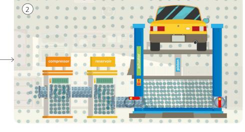
Air is sucked from the atmosphere and squashed in a compressor. The compressed air is stored under high pressure in a reservoir. When the in valve between the reservoir and the actuator is closed, air cannot move out of the reservoir and the piston remains down.
